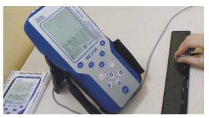
Sondicator technology uses a dual element piezoelectric transducer to transmite and receive sound waves into composite materials. Any disbond or delamination within the inspection zone attenuate the sound waves and an experienced technician can interpret and determine the location and relative size of the disbond condition.
