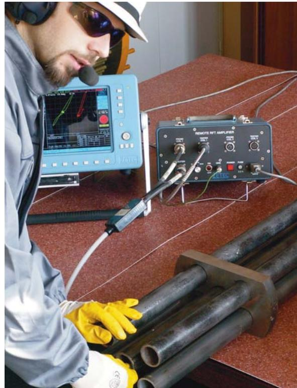
Evaluating the quality of products by Remote Field Testing method is the most effective for ferromagnetic materials like low carbon steels, chrome molly, duplex in units like:
