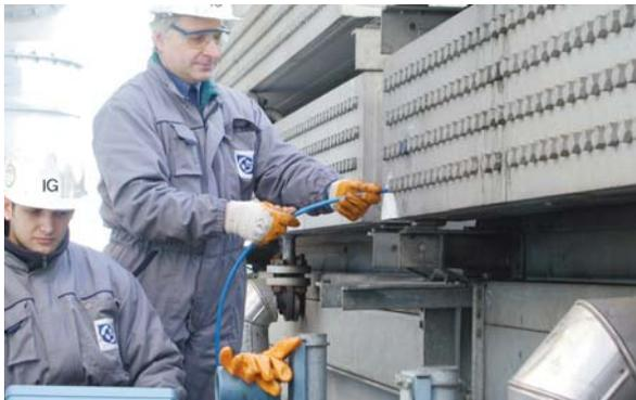
RFT can be used to inspect any conducting tubular product, but is generally considered to be less sensitive than conventional current techniques when inspecting non-ferromagnetic materials.
